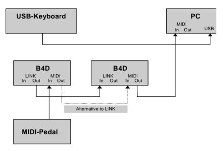
In this example a keyboard is connected to the USB port of the PC. Another B4D is added to the systen, so that you are able to control the drawbars for the upper and lower manual directly without switching. Therefore, you can either use the provided MIDI cable or a Link cable. Using a Link cable just one power supply unit is neccessary since the power supply takes place across the Link cable.
