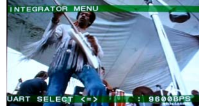
C. Down (V) key then Left or Right keys to set the desired Baud Rate.
