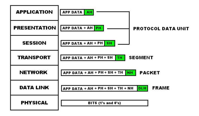
As data is processed first down through the model a packet is built, eventually it contains several headers and the original data resides in the middle known as the payload and the end of the packet has a trailer which may contain information that validates the packet. The trailer often contains a CRC and if the CRC is not matched at the destination end, the entire packet will be discarded and a request for a new one is sent.
