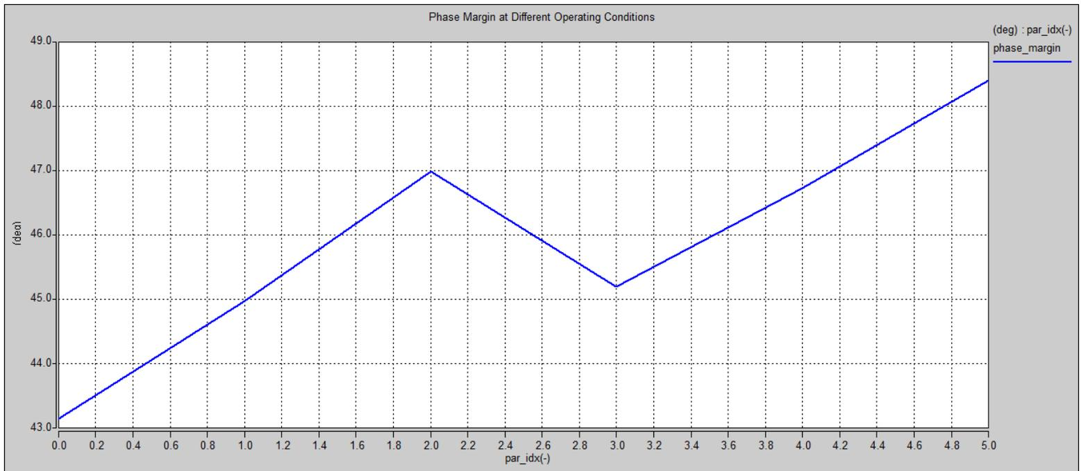
**Figure 9:** Phase margin measurement of the overall open-loop transfer function
