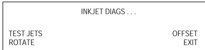
3. Press **F1**-Test Jets to display the Test Jets menu.
