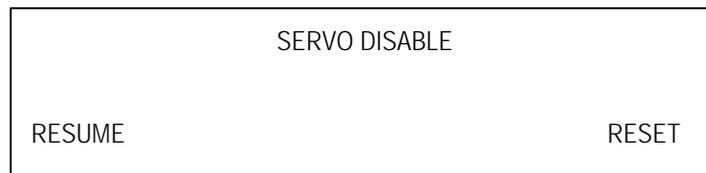
Disabling the servos does not remove power to the plotter. All plot and position data is kept intact.
