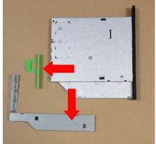
**2.4** Stabbing into a small hole on the ODD bezel with a pin to ejecting the ODD tray then pull the ODD bezel to separate it from the tray.
