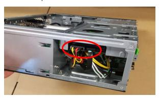
**4.2** Remove two screws fastening HDD cage
