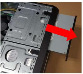
2.3 Remove two screws at the back of ODD to disassemble the ODD brackets
