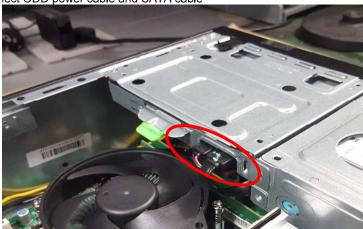
2.2 Press the tail of ODD to pushing it out of chassis
