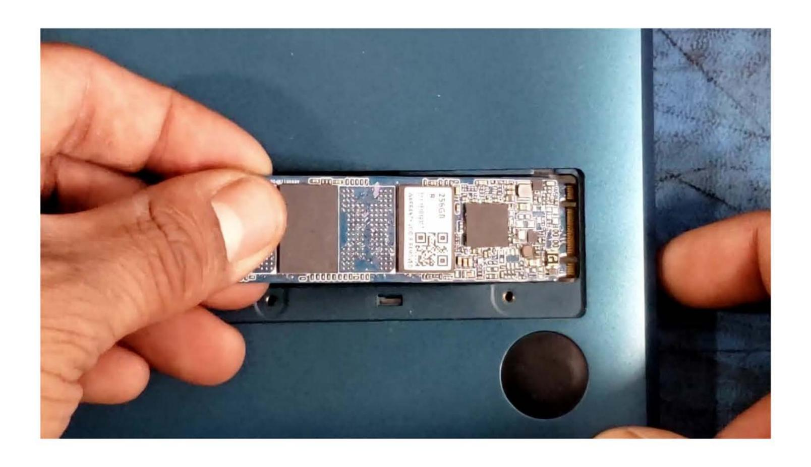
4) Use the screw we removed in step 2 to screw down the other side of the SSD down.
