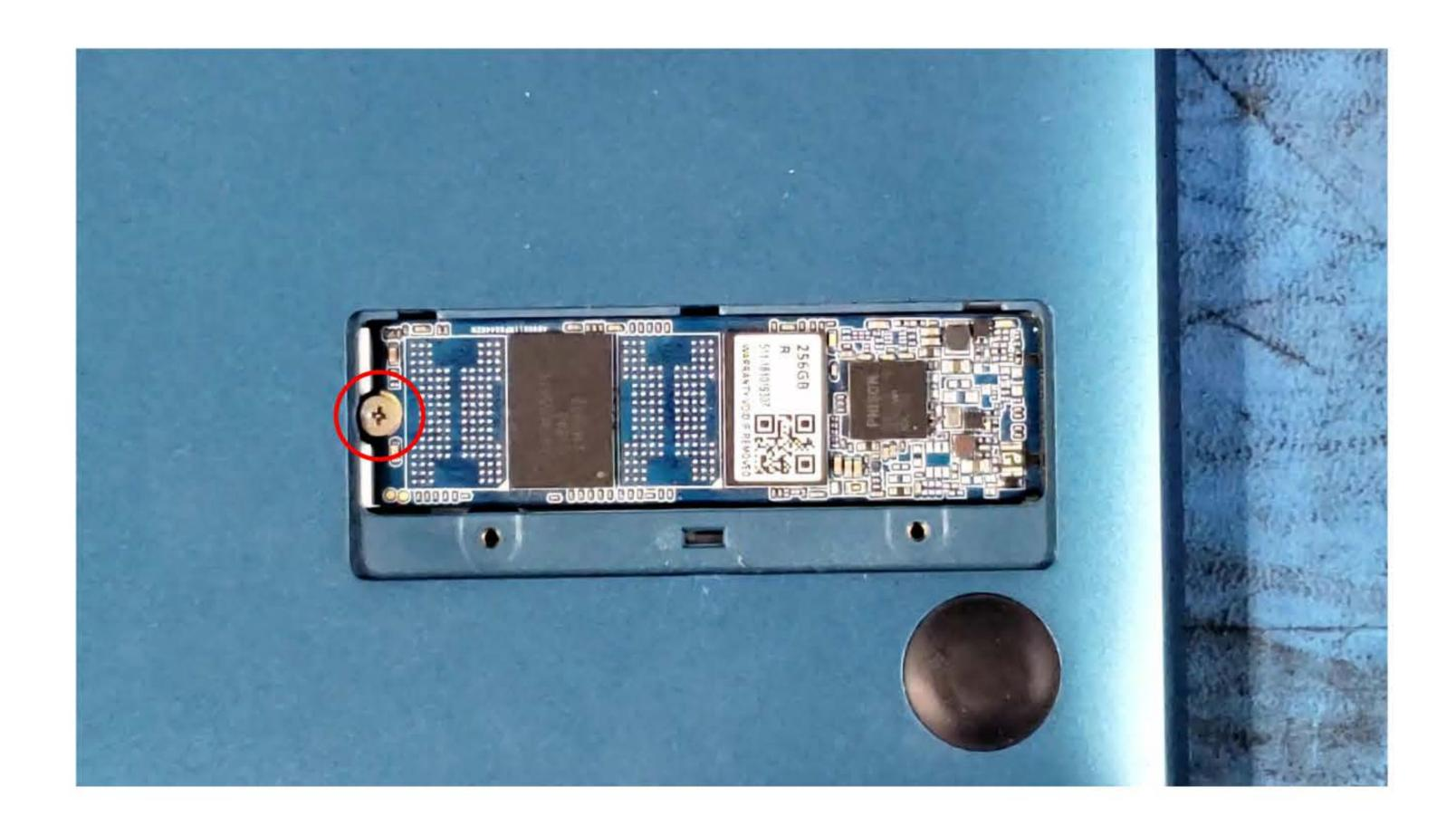
5) Insert the SSD cover and screw it back in using the screws we removed in step 1.
