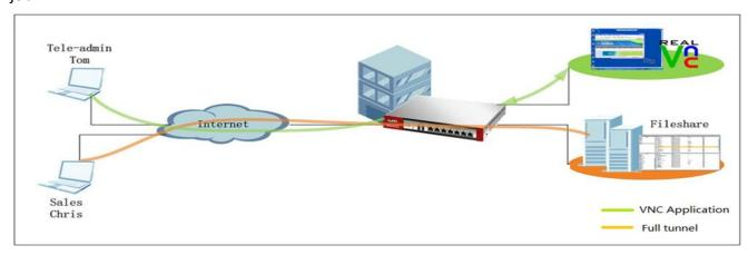
**NOTE:** USG 50 supports RDP, VNC, WEB link application and SSL VPN full tunnel, but doesn't support SSL VPN file-share and OWA applications so far. If the remote clients want to use file-share and OWA through SSL VPN, they can use SSL VPN full tunnel mode (Security Extender) as a workaround.
