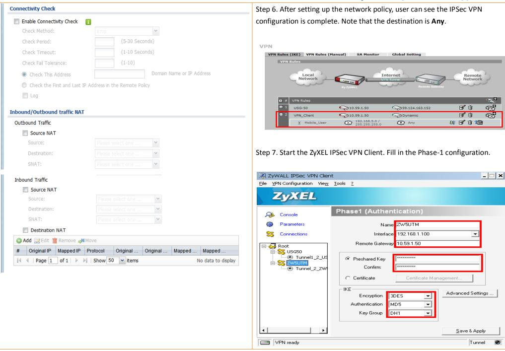
Step 7. Start the ZyXEL IPSec VPN Client. Fill in the Phase-1 configuration. Note that the USG series does not support the "Config Mode" in phase-1 advanced setting, thus users must avoid selecting it when performing configuration.
