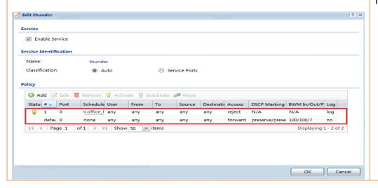
Step 3. IDP signature update. To keep the ZyWALL IDP engine performing at its best, make sure the IDP signatures are kept updated (The **update** procedure can be done manually or automatically.)
