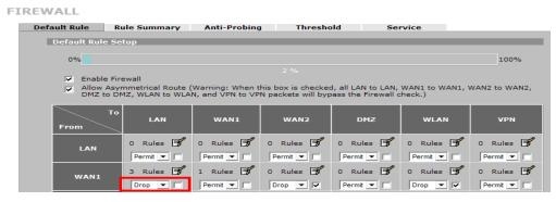
Step 4. Click **CONFIGURATION > Network > Firewall** to open the firewall configuration screen.
