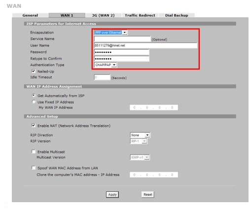
Step 4. Enable the interface and select the pre-configured ISP account to activate the PPPoE rule.
