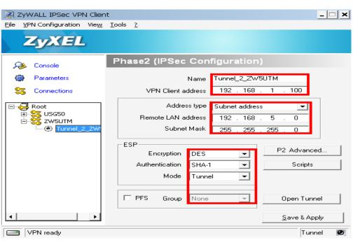
Step 8. Configure the phase-2 parameters.
