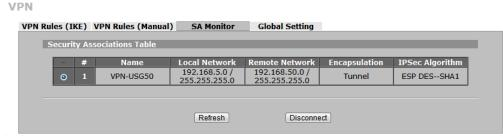
Step 7. After setting the rule, user can select the rule and click the **Connect** button to establish the VPN link. Once the tunnel is established, a **connected** icon will be displayed in front of the rule.
