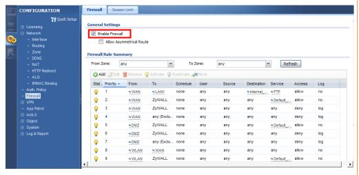
Step 5. Click the Add button to create a firewall rule to enable the FTP service to pass from WAN to LAN1.
