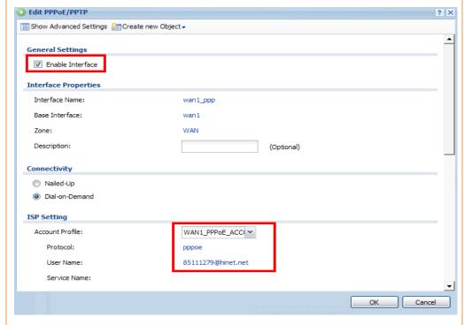
Step 5. When the configuration is done, click the **Connect** button to enable the PPPoE link. Once the connection is established, the *connected* icon will be displayed in front of the rule.
