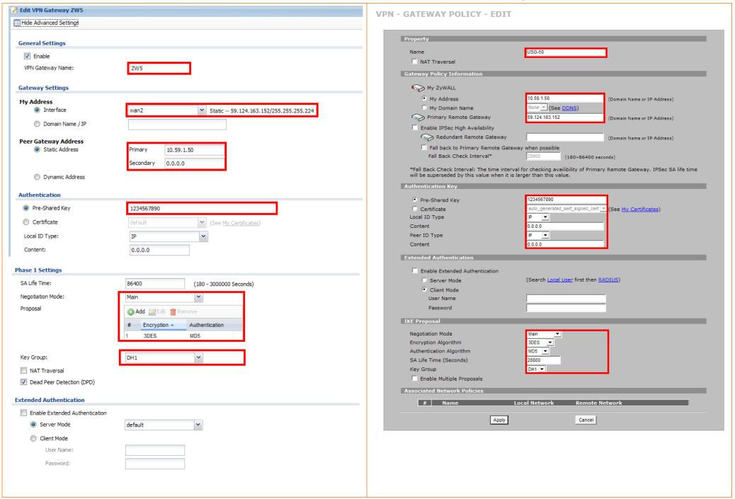
Step 4. Click **CONFIGURATION > VPN > IPSec VPN > VPN Connection** to open the configuration screen to configure the phase-2 rule.
