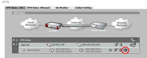
Step 7. After the VPN tunnel is established, user can find the SA information on **SECURITY > VPN > SA Monitor**.
