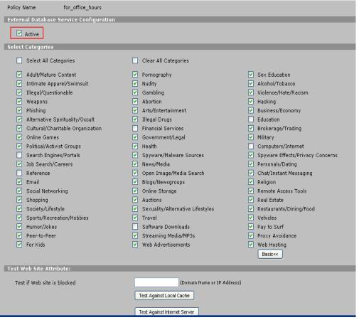
Step 4. Switch to **Configuration > Anti-X > Content Filter > General**. Enable **Content Filter**.
