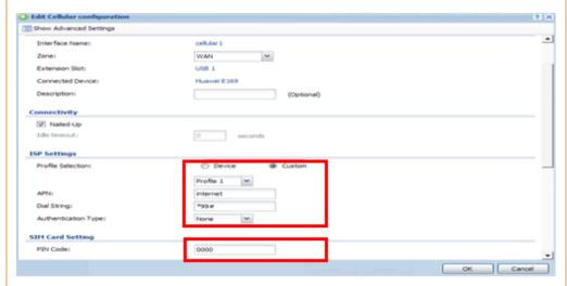
Step 9. After the configuration is done, click **Activate** to enable the rule. And then click Connect button to enable the 3G connection.
