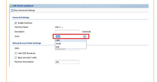
Step 2. Configure the WLAN bridge to the LAN zone. This will give the WLAN users the same security properties with the LAN server.
