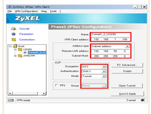
Step 9. Because it is a dynamic rule, user MUST enable it from the VPN client. Click **Open Tunnel** to enable it. The icon will change to green if established successfully.
