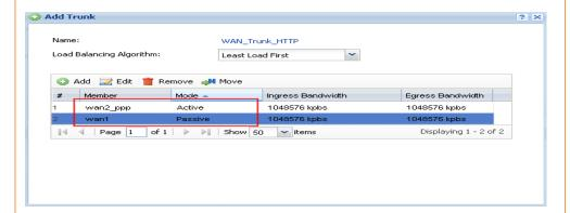
Use SYSTEM\_DEFAULT\_WAN\_TRUNK to do load balancing for all other traffic.
