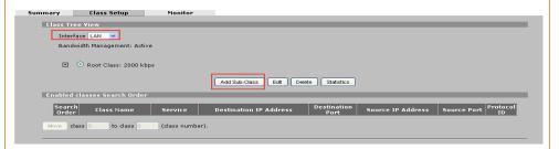
To guarantee voice quality, the bandwidth for VoIP traffic with should be at least 300Kbps in both download and upload directions.
