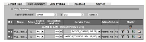
Step 6. Configure the firewall rule to enable the FTP service to pass from WAN1 to LAN.
