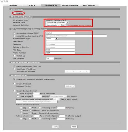
Step 8. Fill in the 3G connection parameters:
