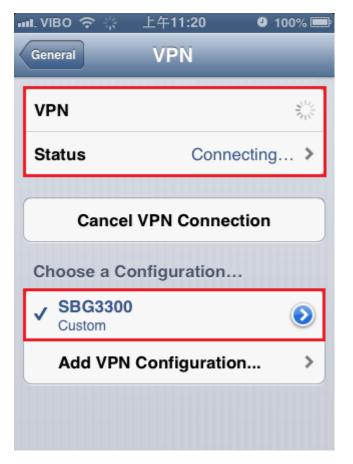
When L2TP VPN tunnel has been connected, the smart phone will show the VPN status on VPN configuration page.
