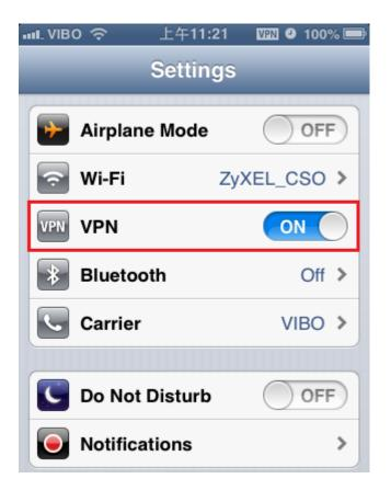
When VPN tunnel has been established, smart phone will display a "VPN" symbol on top information bar.
