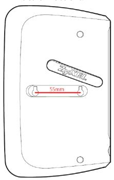
4 Align the holes on the back of the WAP6806 with the screws on the wall. Hang the WAP6806 on the screws.
