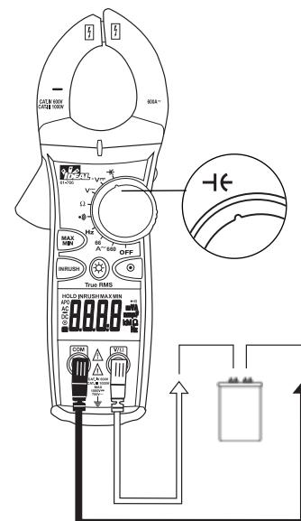
Note: If "disc" is displayed, then voltage exists in capacitor. Discharge capacitor and re-initiate test.
