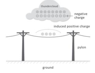
During discharge of the thundercloud (lightning), the positive charge accumulated in the cable is released, resulting in a surge in the cable in both directions.
