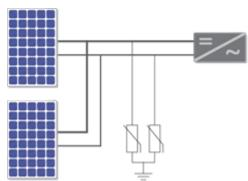
For inverters with an integrated fuse box, internal fuses should be bypassed in order to connect an SPD, and external string fuses should be connected.
