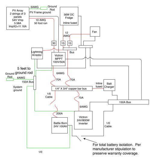
Inverter neutral floated. Utilizing single NEMA plug for the time being. Transition to AC load center later, will bond neutral/ground at that time.
