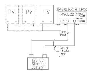
Before mounting the PVCM20 regulator inside the PV panel junction box, clean the surface to which the PVCM20 will be attached. Allow the surface to dry. Remove the backing from the double stick tape and press firmly into box cover.
