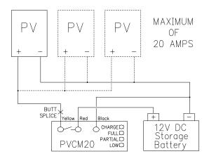
Connect the PVCM20 regulator wires to battery terminals and attach regulator to battery cables with a tie-wrap.
