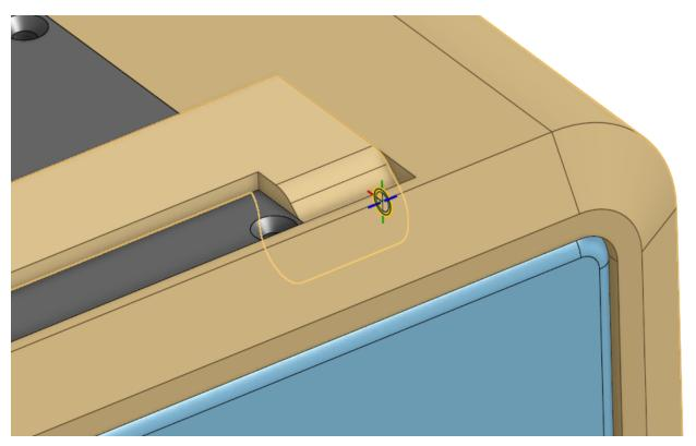
10. Next, let's add limits to the Revolute Mate, so the stand can only open and close 90 degrees. Use the Play button, , to ensure the direction and limits are correct (click on "Reorient secondary axis" until the direction of rotation is correct):
