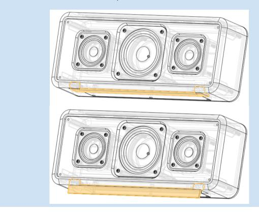
8. Let's start by assembling the stand. We want to be able to swing open the stand to prop the speaker up. Turn the model upside down, and click on the stand. Use the triad to translate it out of place just a bit (this will expose the surfaces we will use for referencing the Mate Connectors):
