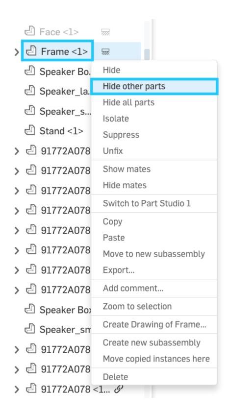
30. Navigate to the Frame part in the Parts List, expand it, and unhide our "Battery Mate Connector". This will make it easy to select:
