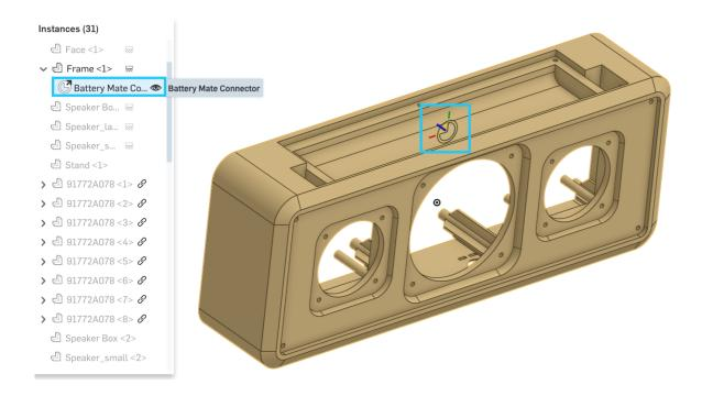
31. Now, make sure Snap Mode is on, and insert the battery part:
