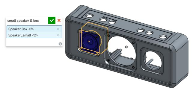
18. Now, you may move this group using the triad, and notice how the speaker and speaker box stay in the same position relative to each other. Unhide the other parts, and we should now have an assembly that looks like this:
