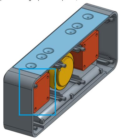
21. Once again, using Snap Mode, assemble 4 button head screws to the second small speaker:
