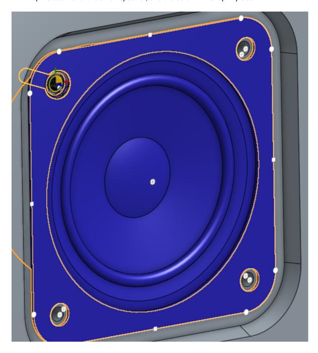
Pro Tip: Remember when we used the [Shift] key on the keyboard to lock into the current geometry selection in the Cantilever Clamp in Lesson 4? It would help to do so here; hover over the front face of the speaker, and hold [Shift] to see all the inferred Mate Connector locations:
