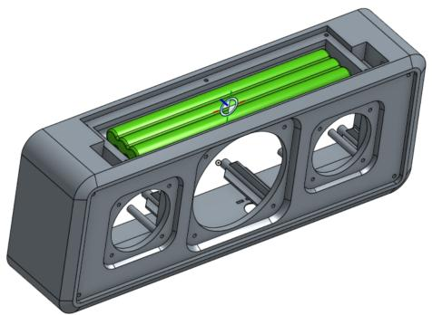
34. Next, unhide our battery cover, and assemble a flathead screw into one of the chamfered holes:
