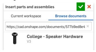
12. Select the document, and then select the button head screw. Now, as you hover over the model, Onshape is automatically "waking up inferred Mate Connectors". Hover over the Top-Left corner of the small speaker, and the screw will snap in place:
