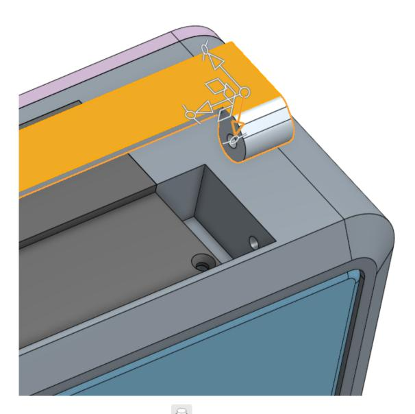
9. Next, create a revolute mate, by referencing the pin holes in the Stand and in the Frame:
