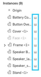
**Design Intent Check**: We want our stand to swing open to prop the speaker up. How should we mate the stand to the rest of the speaker? What should the limits be?
