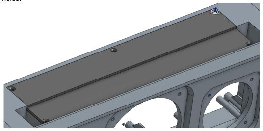
35. Next, Replicate the screw to the rest of the holes in the cover, by referencing both faces:
