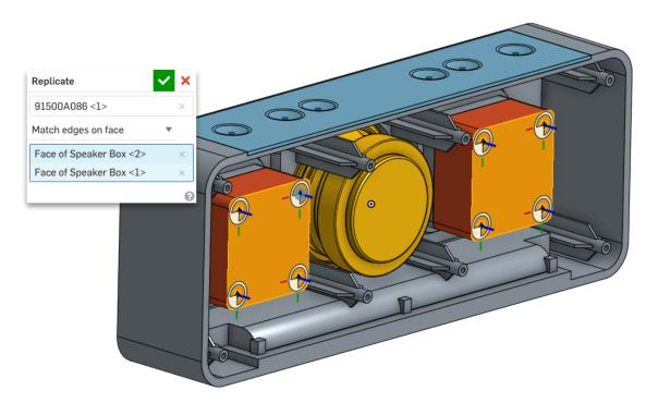
24. Click the Green checkbox. Since all the circular edges (holes) in the two speaker boxes are identical, the Replicate tool will automatically add and mate the flathead screws to the remaining holes. There should be seven more instance of the flathead screw in our Parts List, and there should be seven more fastened Mates:
