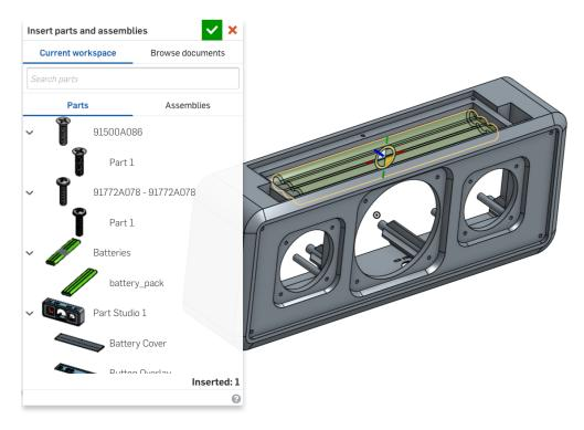
33. Now, just click the screen with the left mouse button, and the batteries will be dropped in place:
