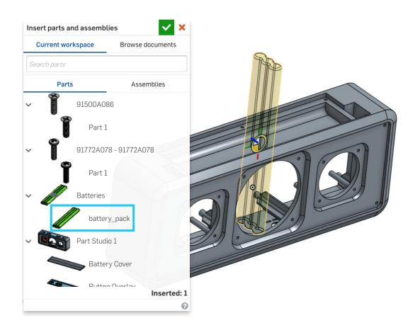
32. In this case, our batteries are rotated 90 degrees by default (this is due to the orientation of the green and red axis on the Mate Connector). Before clicking, rotate your batteries while in Snap Mode using the "q" key:
