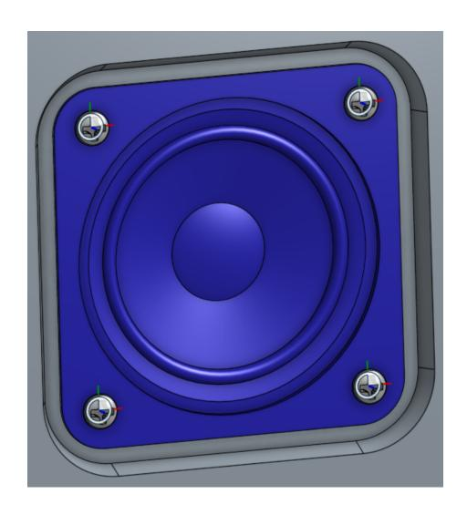
15. Next, let's continue using Snap Mode to assemble the same screw to the large speaker:
