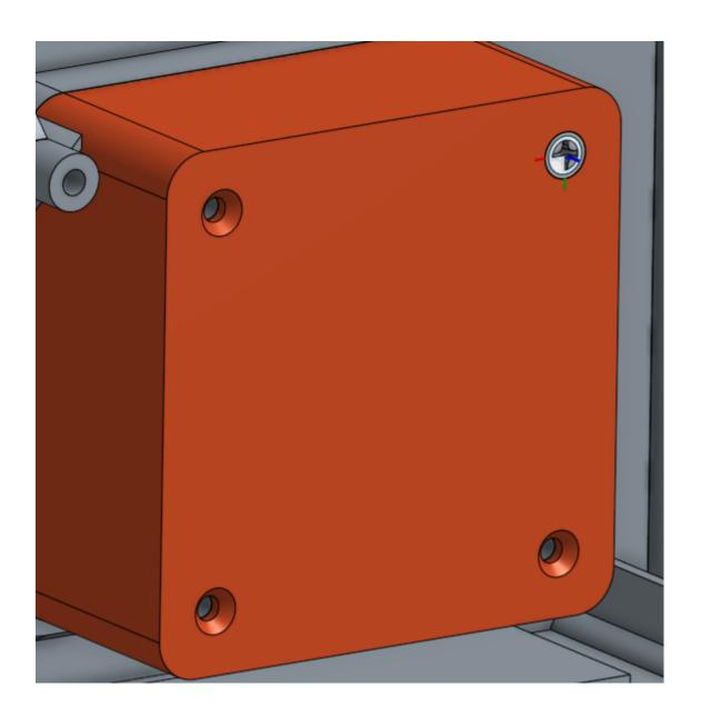
23. Next, select the Replicate tool, . Use the flathead screw as the "seed instance", and select the faces of both speaker boxes as the reference face:
