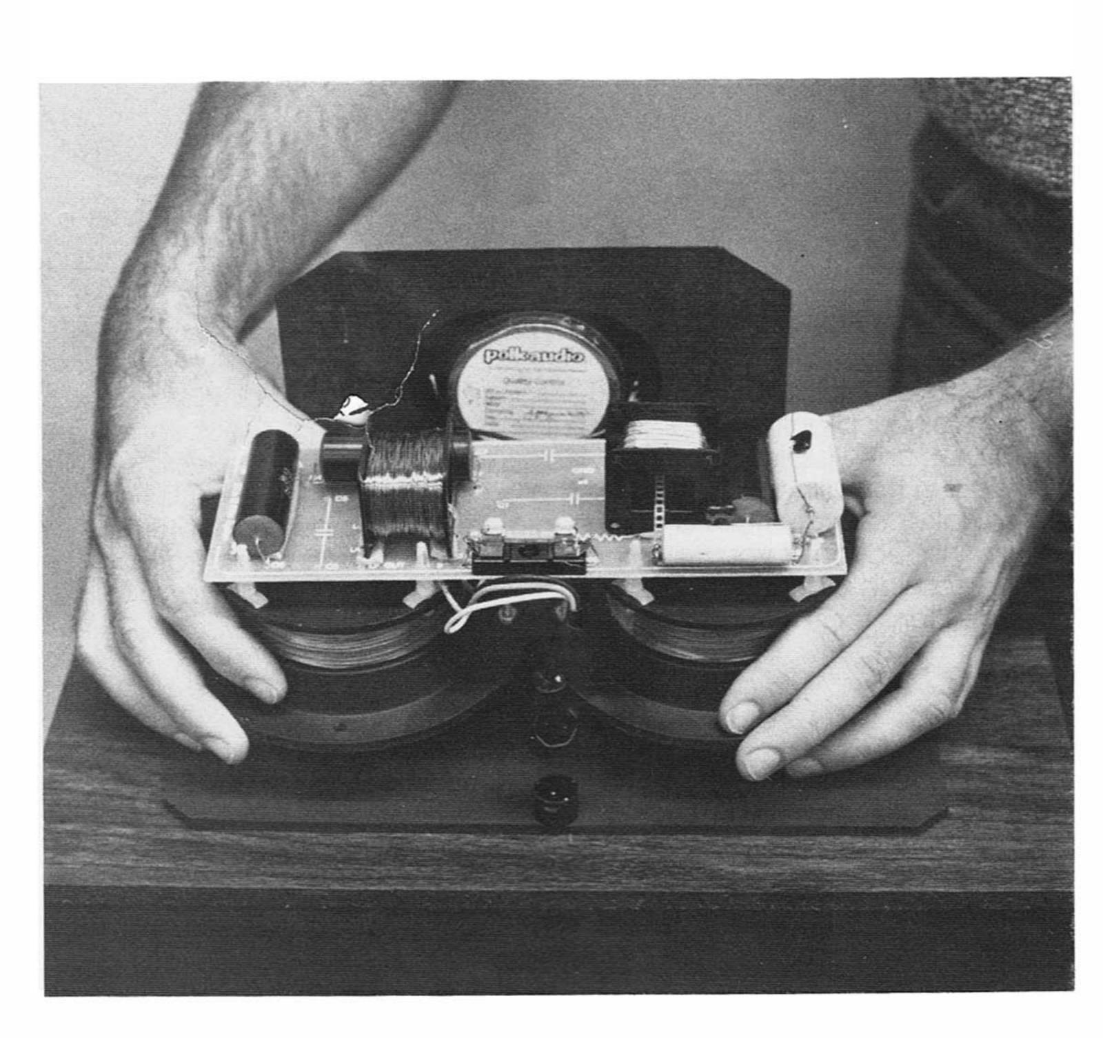
4. The High Frequency Modules are identical and can be placed on either cabinet. Place the modules on the cabinets so that the outermost hole on each side fits over the threaded stud. Replace the thumb-nuts finger tight. Do not overtighten.
