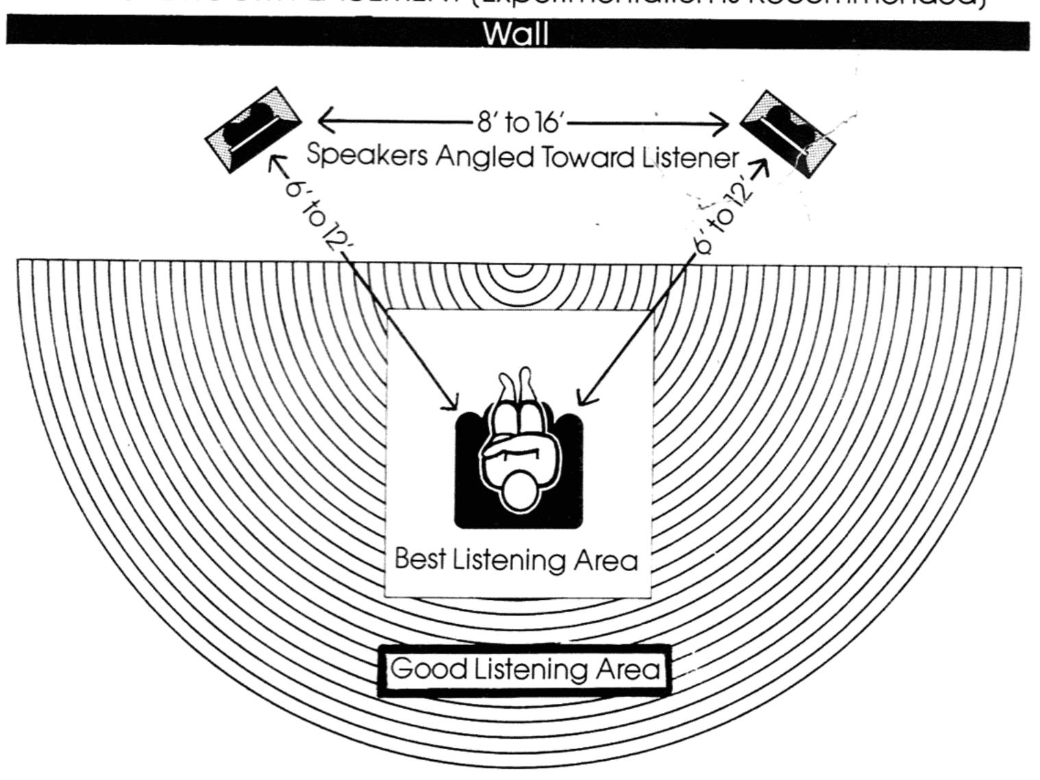
Both stereo imaging and sonic balance can be influenced by room position. Best sonic balance will usually occur when the speakers are placed far from the corners and at least 3 feet from other walls. Placement near or in corners will emphasize bass response, while placement close to or against walls will emphasize lower midrange.
