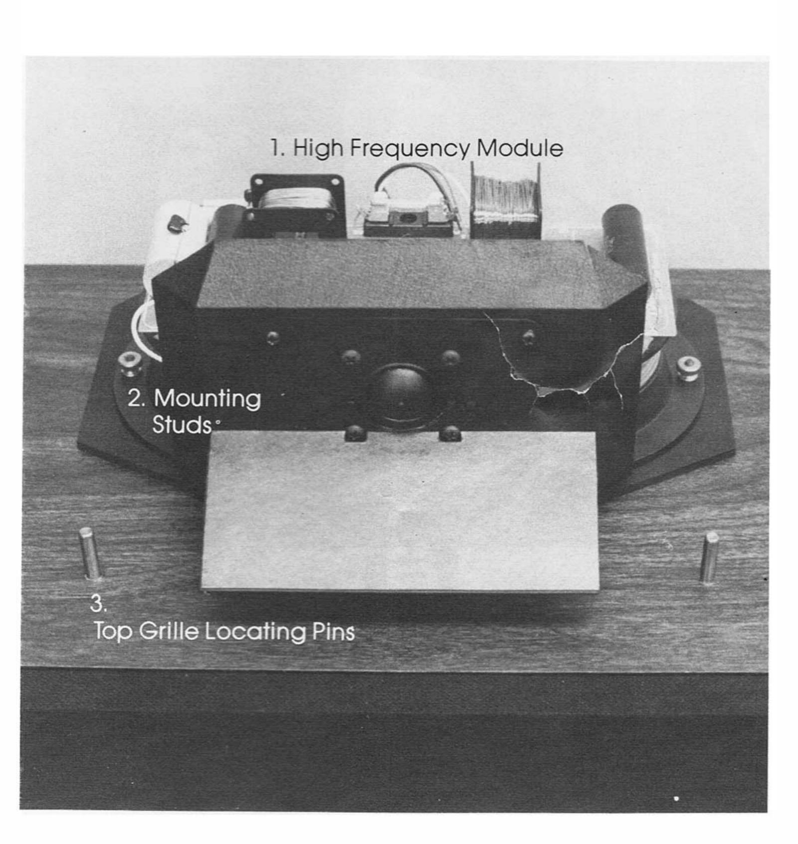
5. Look at the connector at the back of the High Frequency Module. It has three ridges to guide it into the socket on the cabinet. Rotate the connector to align the ridges correctly and press gently into the socket until it locks into place. (To remove, squeeze the ridged sides of the connector hard and lift. Do not attempt to force it.)
