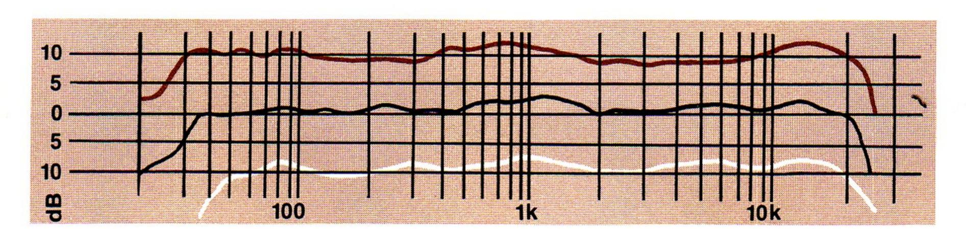
On-axis response in controlled reverberant field environment. Curves are offset 10 dB for clarity of presentation.
