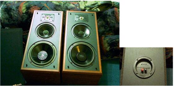
Subwoofer 1 - 8" Diameter fluid coupled subwoofer (sub bass radiator) Midrange 1 - 6-1/2" Diameter (16.51cm) drivers MW6502 Tweeter 1 - 1" Diameter (2.54cm) Polk SL2000 silver coil dome tweeter
