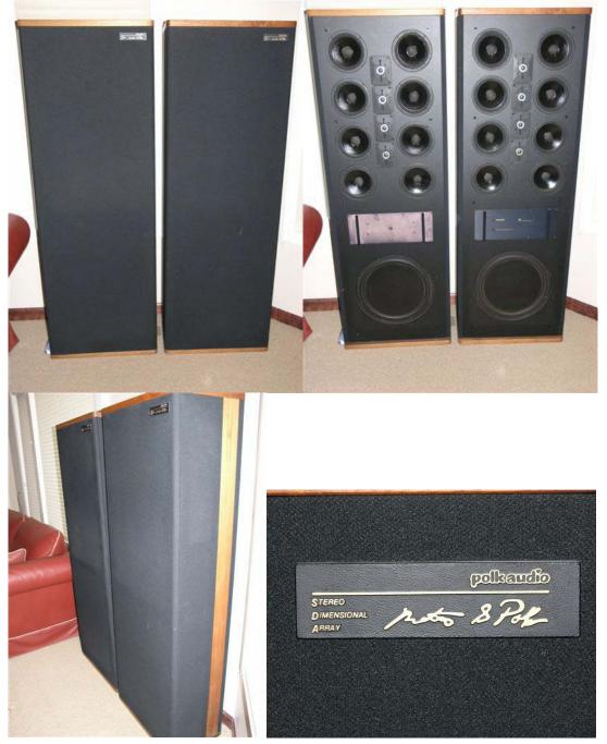
Subwoofer 1 - 15" Diameter (38.10cm) Sub-bass radiator Midrange 8 - 6-1/2" Diameter (16.51cm) Trilaminate-polymer drivers (MW6503) Tweeter 4 - 1" Diameter (2.54cm) SL2000 Silver Coil dome tweeters
