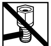
Do not insert insulated section of speaker wire
