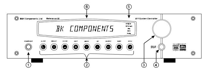
**1. Headphone Jack** - Stereo headphones having a standard ¼ inch binaural plug can be connected to the headphone output. The processor must be on and in HEADPHONE Mode for proper headphone operation.
