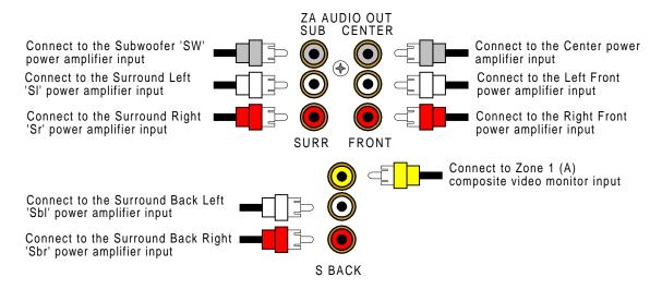
**Subwoofer Output -** Connect an RCA cable from the processor's SW output (part of the surround outputs). If your subwoofer does not contain its own amplifier you will need to purchase an external B&K or other power amplifier. Connect the processor's SW output to the audio input of the external amplifier. Connect the external amplifier's speaker output to your subwoofer.
