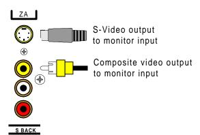
**Video Monitor** - Attach one end of the composite video interconnect cable to the video input on the monitor, then attach the other end to the yellow video output on the processor's ZONE OUTPUTS. Repeat for the S-video connections if you are using S-video. Dual zone operation requires connections be made to (ZA) for Zone 1, and (ZB) for Zone 2.
