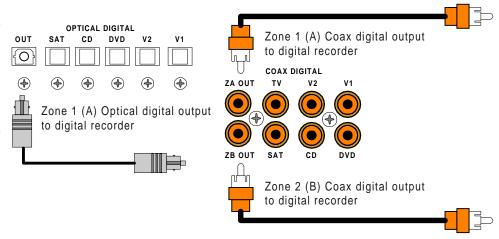
may connect one digital recorder to the optical output and another recorder to the coaxial. Zone 2 (B) digital output is coax.
