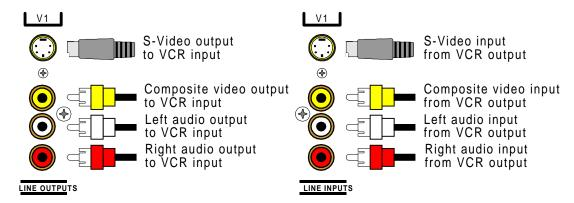
Attach one end of the audio interconnect cable to the left audio output on the VCR, then attach the other end to the left (white) V1 audio input on the processor. Repeat for the right (red) audio connection. Attach one end of the composite video interconnect cable to the composite video output on the VCR, then attach the other end to the yellow video input on the processor labeled V1. Repeat for the S-video connections if you are using S-video.
