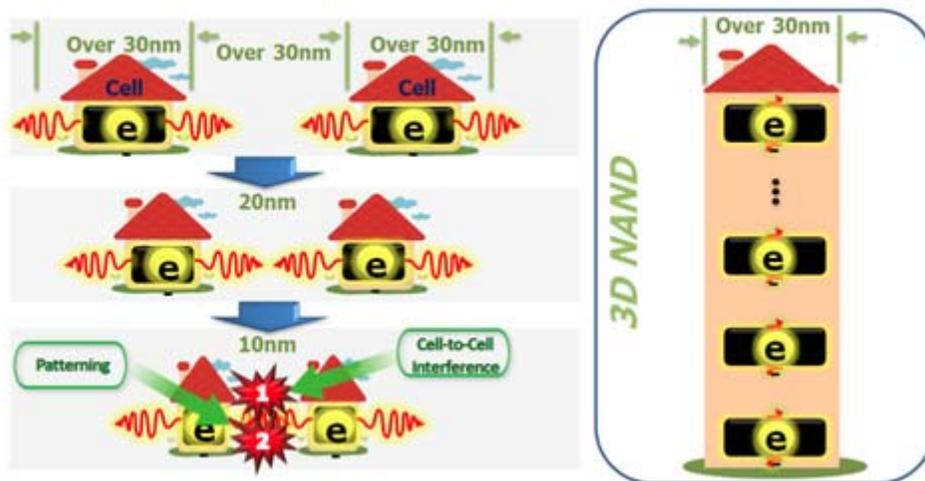
Figure 2.2 Cell-to-cell Interference Mitigated by 3D NAND.
