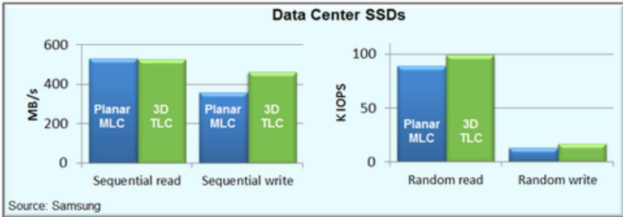
Figure 2.4 Planar MLC vs. 3D TLC SSDs.
