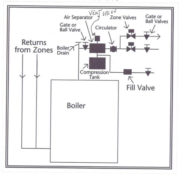
In either case, you'll get rid of your initial air by closing the main service valve and the zone service valves. Next, open the feed valve and the tee-mounted boiler drain. Then, open one zone at a time. It's like firing torpedoes.
