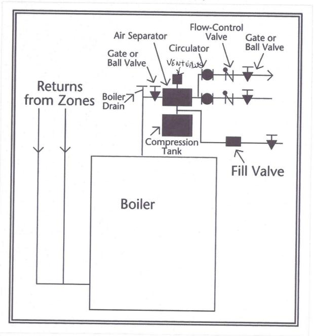
You leave the boiler with a full-size supply main and enter a tee. Pipe a 1/2" boiler drain into the top of the tee. That's going to be the purge valve for your system. You only need one purge valve. You take the money you were going to spend on the other purge valves and you go buy something nice for yourself.
