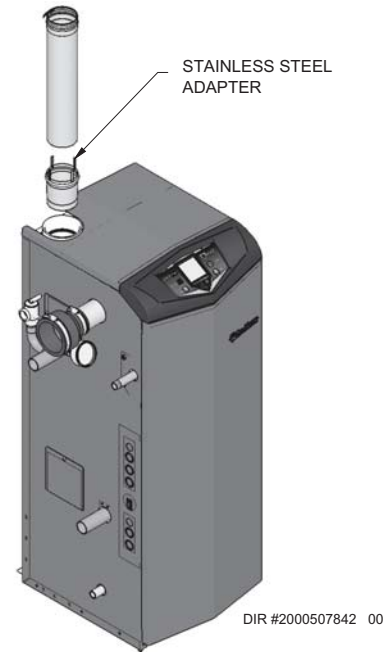
Figure 3-10 Near Boiler Stainless Steel Venting
