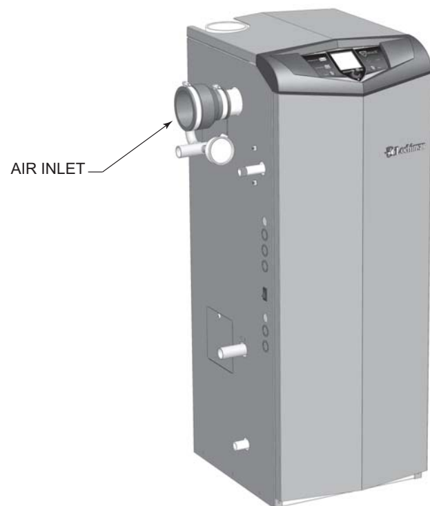
Figure 3-6 Near Boiler Air Piping
