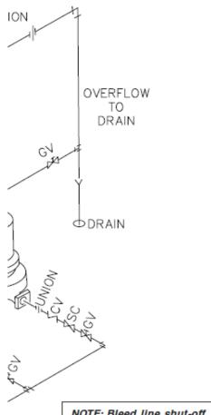
NOTE: Bleed line shut-off valve <u>MUST</u> remain open unless pump is being serviced.
