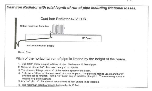
Drawing # 2 shows a cast-iron radiator installed with 1½-inch pipe
