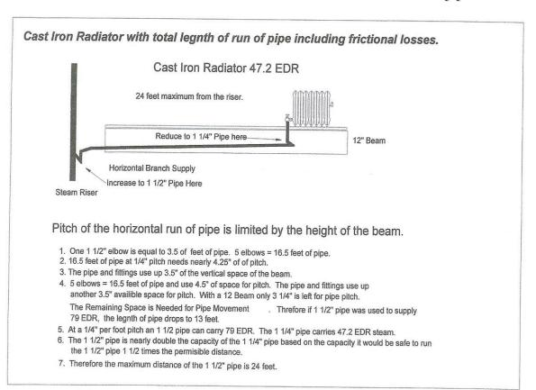
Based on the charts and calculations and what is shown in the drawings, increasing the pipe size of lateral runs to a radiator will permit the radiator to be moved further away from the riser.
