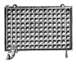
Known popularly as the "mattress type" radiator, this flat box of sheet iron was first patented in the United States by Stephen J. Gold of Cornwall, Connecticut, in 1854. It resembled closely an experimental model invented and built by James Watt in England in 1784. It was never manufactured by H. B. Smith & Co.
