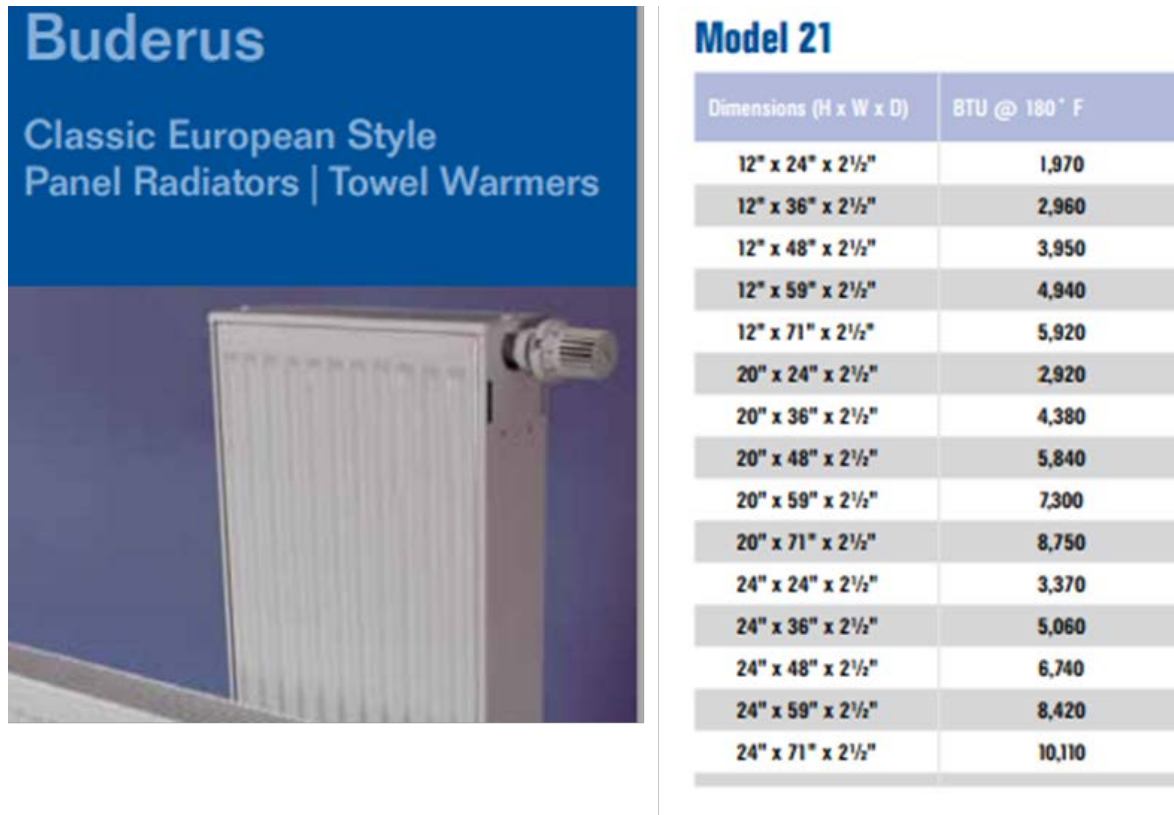
Figure 25. Manufacturer specifications for a modern radiator panel (Bosch Thermotechnology Corp 2010)
