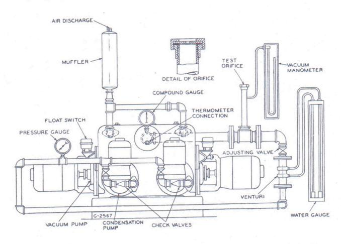
The drawing above shows the factory set-up to test a Nash Jennings Type CSM Vacuum Heating Pump.
