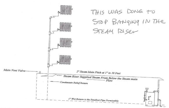
This drawing shows the best way to modify the piping system. The drawing shows a parallel flow steam system with a relief drip at the base of the riser. The difference between both steam systems is how condensate water is handled. Originally, the steam system was a counterflow steam system, where
