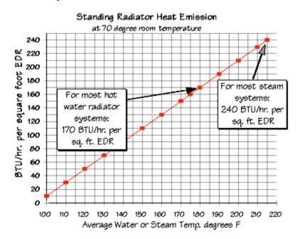
In most cases a Square foot EDR of radiation will emit 240 BTUs per hour on steam heating systems or 170 BTUs per hour on hot water heating systems. This "rule of thumb" proves reliable for cast iron radiators as applied in existing homes in the United States. The above graph shows that these outputs will be higher or lower if the steam or water within them is hotter or cooler. It will also vary if the radiators are exposed to blowers or fans and if they are covered or obstructed.
