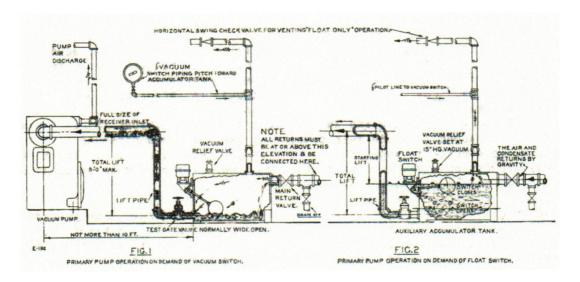
Figure (1) primary pump operation on demand of vacuum switch.
