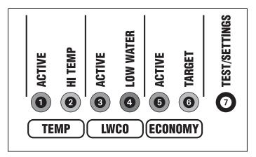
**1TEMPACTIVE** Indicates that the Fuel Smart HydroStat control is powered and that the temperature function is active.
