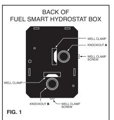
**STEP 2** Place control on the well. While holding box against well nut, tighten well clamp screw. (Fig. 2) **STEP 3** Insert sensor ALL THE WAY into well through the knockout (A or B) you have chosen. (Fig. 3)
