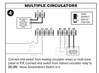
**WARNING** Electrical shock hazard. To prevent electrical shock, death or equipment damage, disconnect power supply before installing or servicing this control.
