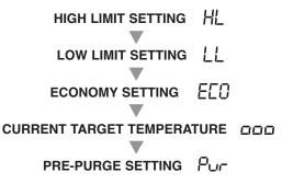
The display will return to boiler temperature (default) if Test/Settings Button in not pressed for 5 seconds.
