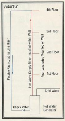
the riser, a passive recirculating line is extended back down to the boiler. This return line could also serve another vertical stack of lavatories; a larger line may be needed to meet fixture flow requirements and not just the needs of recirculating line flow. Note the check valve at the boiler. Without this check valve, the passive recirculating line becomes a parallel hot water supply pipe.
