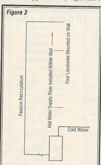
the water heater to the start of the recirculating line under the kitchen sink to cause the thermal now. The main supply piping and the recirculating piping are both 3/4-inch. The branches to each of the four fixtures are 1/2-inch. The drawing is not to scale. but the house is 40 feet long, with the water heater and the kitchen sink at opposite ends. The laundry facility and the two bathrooms are as depicted. To test the system, I timed how long it took at first use for
