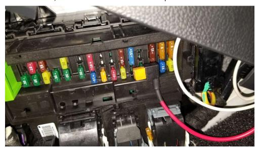
We ran the hot and ground into the engine compartment and attached to the battery positive and negative, with a 30 Amp inline fuse to the hot.
