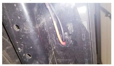
We ran the input wires and the trigger wire along the frame under the truck toward the engine compartment.
