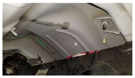
We found a rubber plug in the front passenger footwell and ran the trigger wire into the truck by poking a small hole in that rubber plug. We pulled it out from under the carpet and to the interior fuse panel.
