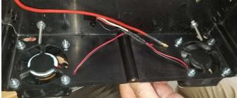
We added a switch to the outside of the box, so that when not towing, the circulation fans won't run.
