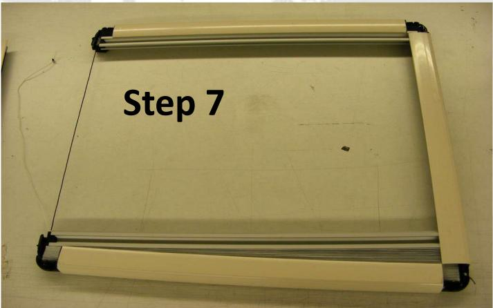
Install the side profiles onto the corner pieces. Repeat this for both sides.
