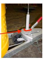
(Fig. 1) Quick release lever; Top-wind jack
