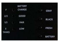
These indicator lights give a general idea of how empty the Fresh, Black or Grey tanks are. For example, pressing the little black button next to GREY causes LED's to appear next to "Empty, 1/3, 2/3 or Full." What you see depends on how the four tank
