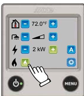
1. Start gas operation by pressing the flame symbol. Gas operation is activated and the flame symbol changes color to green.
