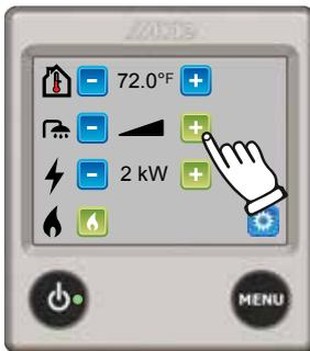
2. **Normal operation.** If hot water is required, press the "+" button (the symbol will then be half-shaded). If the 2.9, section 12 (Floor heating\*) function has been set to Cont., this option cannot be selected. When only hot water is required, e.g., during the summer or when no heating is needed, no settings need to be made; the heating system handles this function automatically.
