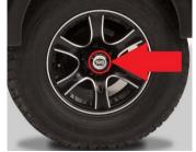
says T@B shown inside the red circle in the adjacent photo. If the temperature readings between drivers & passengers side differs by more than 30-degrees, the bearing may be in trouble.
