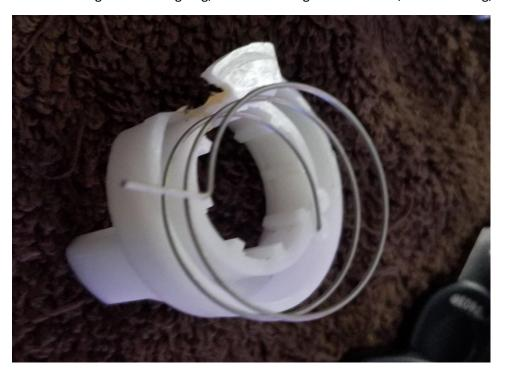
The spring has an "L" that goes into a hole in the white ring.
