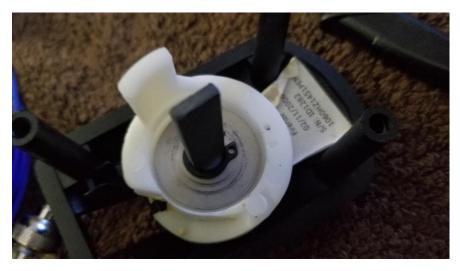
After removing the retaining ring, remove the large silver washer, the white ring, and the spring.
