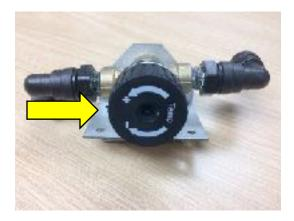
After you have turned the knob twice to the max setting remove the knob and place it back on half way between the + and - so it will be in the position shown to the left. Now you will want to reinstall the screw. This position should be 109 degrees, turning to max of 118 and minimum of 100 degrees. This is how the valve is calibrated from the vender.
