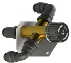
The 3102-002 mixing valve should have a max water temperature output at the valve of 118 degrees. This will give you a temperature at the shower of 108 -113 degrees. The average person takes a 102-104 degree shower. If the water temperature, while on max hot, at the shower faucet is lower than 105 degrees you will need to adjust the mixing valve. The following steps will show you how to adjust the mixing valve if it is on max and not getting a high enough temperature at the shower.
