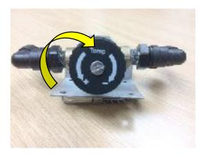
A ¼ turn will put the knob in this position, you can make this adjustment only twice. If it would need to be adjusted up more the valve should be replaced.
