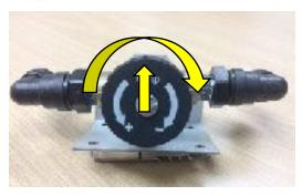
Start by turning the valve clockwise all the way to the lowest (minus -) setting. Take the center screw out of the knob and pull the knob off, reinstall the knob just past the stopping point and keep turning until it stops (bottoms out)
