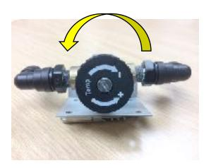
If the valve is still not letting enough hot water at the shower faucet while at the max setting adjust the valve by turning it to the max stop, Remove the screw and put the knob back on a ¼ turn from the max setting.
