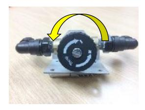
Reinstall the knob back on to the lowest setting and then turn it counter clockwise till it hits the max stop position. Jump the knob over the stop and turn it again counter clockwise till it hits the stop again. This will be two complete turns of the valve.
