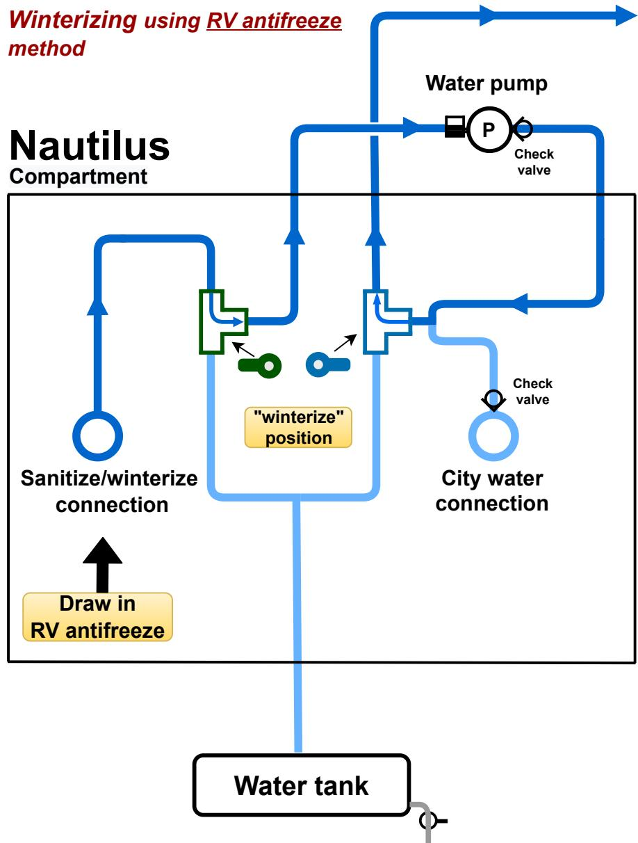
**NOTE:** First set valves to the 45 degree position to blow out Nautilus harness (area behind the Nautilus panel), then set to "Winterize" position to blow out the lines.
