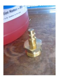
This is a "blow out" plug that fits into your city water connection, then connects to a standard air compressor hose... KEEP THE PRESSURE WELL
