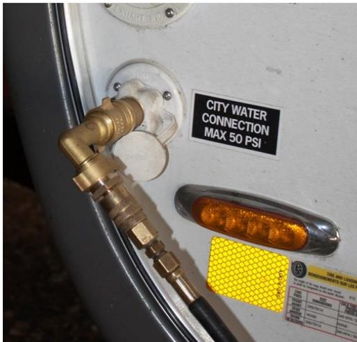
**Air compressor hook up.** Here the standard water pressure regulator is screwed into the city water connection; a right angle adapter is next, followed by the air adapter and finally the air hose.
