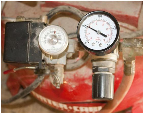
Air compressor set up. Supply tank pressure on the left gauge, output pressure controlled by knob below on the right.
