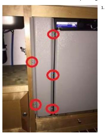
Remove the screws from the 3-way refrigerator side panel that are circled.
