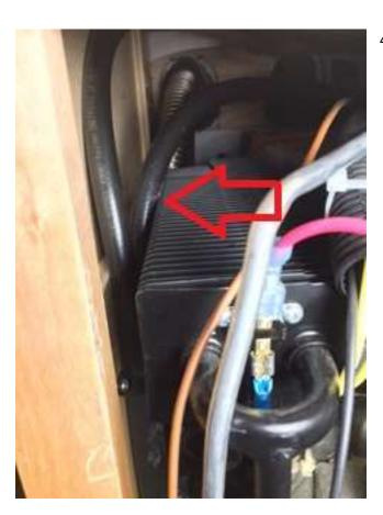
4. This is an example of the <u>improper</u> installation of the gas hose and clips. The gas hose is rubbing against the fins of the 3-way refrigerator.
