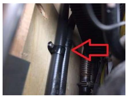
5. This is an example of the improper installation of the gas hose clips.
