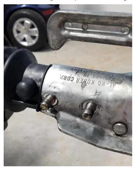
9. Work the front of the bellows over the rear bolt.
