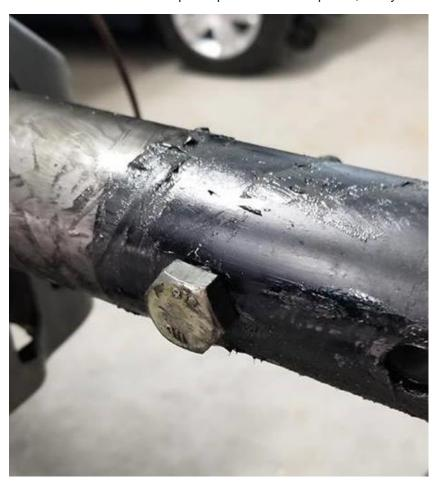
7. Slide the bellows over the piston and behind the bolt you have in there.
