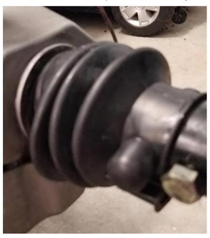
8. Remove the bolt, then, as quickly as possible put the hitch back on the piston. Using a screwdriver to align the holes put the bolts back in through the hitch. Then tighten the nuts.
