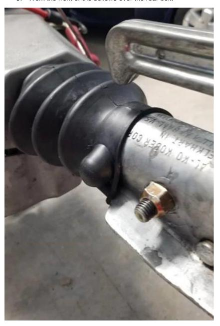
10. Then raise up the front of the plastic cover and work the rear of the bellows over the circle rim, then snap the plastic cover back down.
