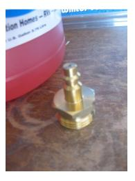
This is a "blow out" plug that fits into your city water connection, then connects to a standard air compressor hose... KEEP THE PRESSURE WELL BELOW 50psi!
