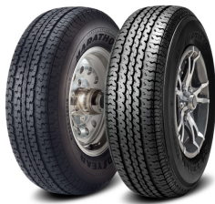
ST (Special Trailer) tires, like these from Goodyear and Maxxis, are available for travel trailers and fifth-wheels, as well as folding campers.
