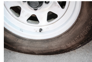
Old tires with visible cracking should be replaced to avoid failures.
