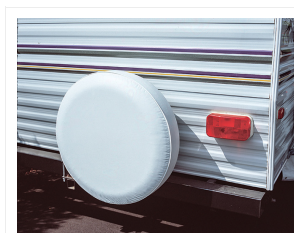
Spare-tire covers can help extend the useful life of the rubber by keeping the sunlight off.
