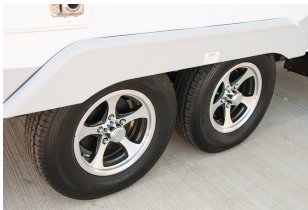
When trailer tires fail, they often damage surrounding fender skirts, sidewalls, wheel wells and trim. Note that these tires are filled with nitrogen, indicated by green valve caps.
