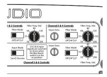
1) "Filter Mode" Control: The M6600 employs a 12dB per octave filter for each pair of channels (one filter for channels 1&2, another filter for channels 3&4 and a third filter for channels 5&6). Each of these filters can be configured independently into one of two filter types or defeated completely by way of the three-position "Filter Mode" switches:
