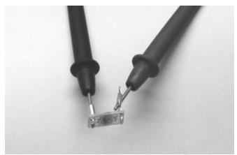
Figure 5.0 - Thermostat Resistor
